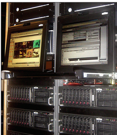
The Discovery Channel uses a 32-channel system for monitoring and logging, with eight Observers (which are located at the bottom of the rack) and one WEB/SQL server (not shown). Photo courtesy of Discovery Channel.
